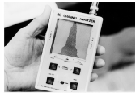
Here the analyzer is set to look at the entire 72 to 73 MHz portion of our R/C band. In this particular photo there are two R/C channels on the air (above left), the one to the left is Ch 44, the other Ch 56. A typical display of an R/C transmitter which is clearly narrow band (above right). Dr. Walt Good (C) confers (below) with Terry Good (L) and Mrs. Dale Mulholland during a SAM meet at the Odessa field.
