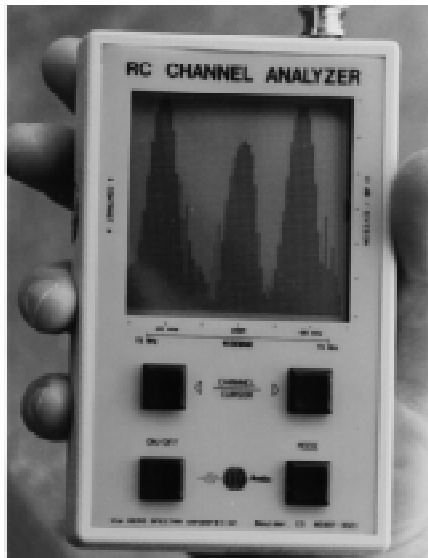
The Channel Analyzer can operate in its first mode as a frequency scanner scanning for all signals in the 71.9 to 73.1 MHz bands (above left). In second mode (above right) it scans for adjacent channel interference.
