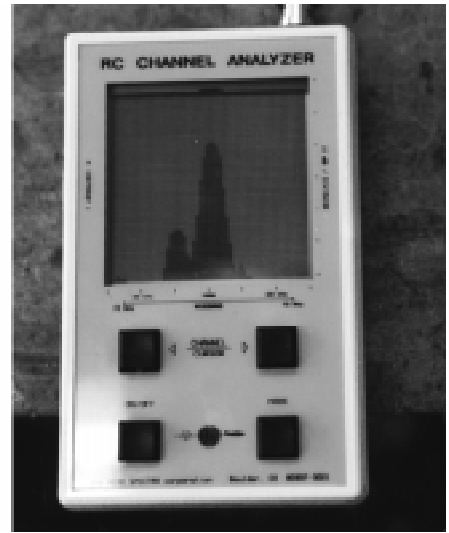
Operating in its second mode as a spectrum analyzer, the screen displays a signal that exhibits a signal with good narrow modulation (above left) with the signal within \pm 6 KHz. This screen (above right) displays a pager signal 10 KHz away from an R/C signal (the larger node).
