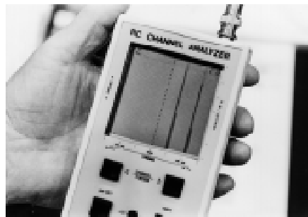
Here the analyzer is set to look at the entire 72 to 73 MHz portion of our R/C band. In this particular photo there are two R/C channels on the air (above left), the one to the left is Ch 44, the other Ch 56. A typical display of an R/C transmitter which is clearly narrow band (above right). Dr. Walt Good (C) confers (below) with Terry Good (L) and Mrs. Dale Mulholland during a SAM meet at the Odessa field.
