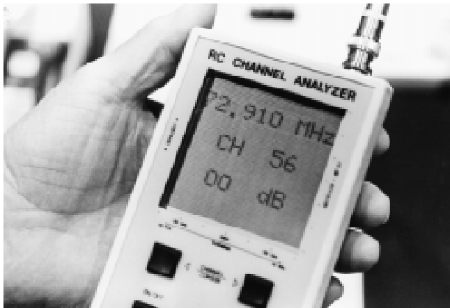
Among the choice of display information, the Analyzer's third mode shows frequency, channel number, and signal strength (above left). As Terry Good (R)
